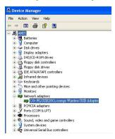
4. Verify that the device status of CG-WLUSB2GO is [This device is working properly]->Click [OK] to close this page.
